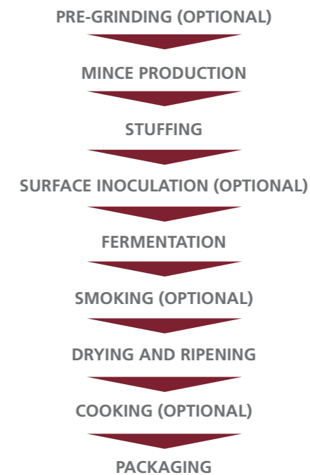
Figure 1. General flow diagram of sausage production
